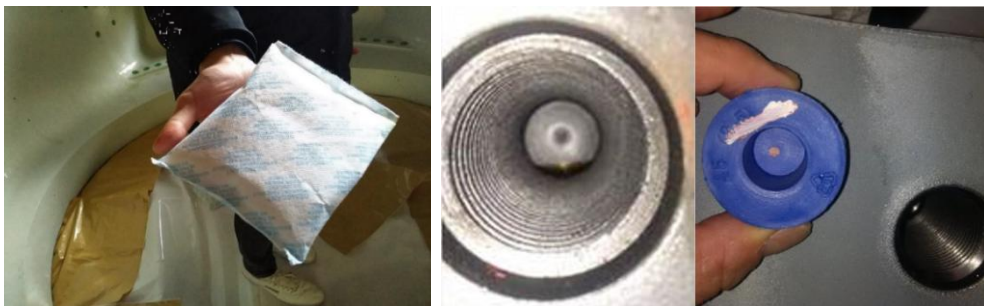
Figure 1: Example for desiccant bag (l.) and bore hole protection (r.)
