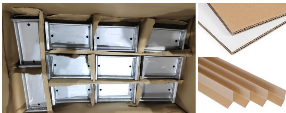
Figure 2: Example for spacer between components and edge protections
