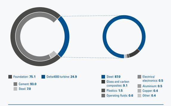
The size of the tower foundation depends on different influencing factors such as the type of soil and the height of the water table. At 87% steel is the dominant material in the material mix of the Delta4000 turbine with a 105 m tower, without the foundation. At 49 t, glass-fiber and carbon-fiber reinforced composites are the second-largest materials group.
